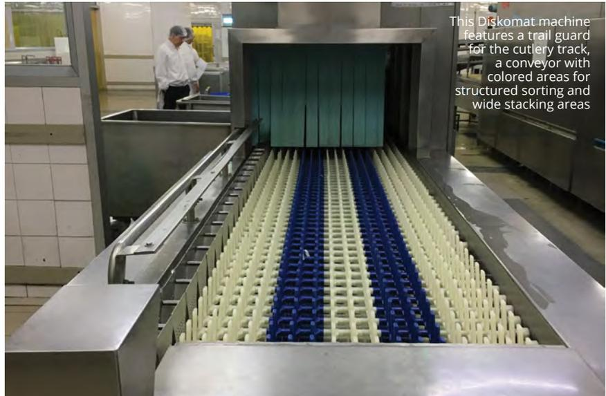
This Diskomat machine features a trail guard for the cutlery track, a conveyor with colored areas for structured sorting and wide stacking areas
